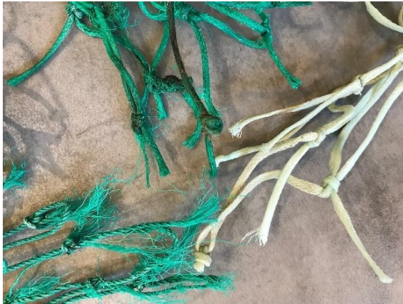
Figure 2. Fragments of trawl net were examined and appeared to be cut rather than ripped.
